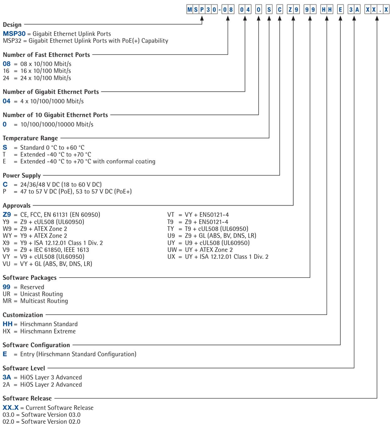
**NOTE:** The last four categories (**Customization, Software Configuration, Software Level** and **Software Release**) are optional.
