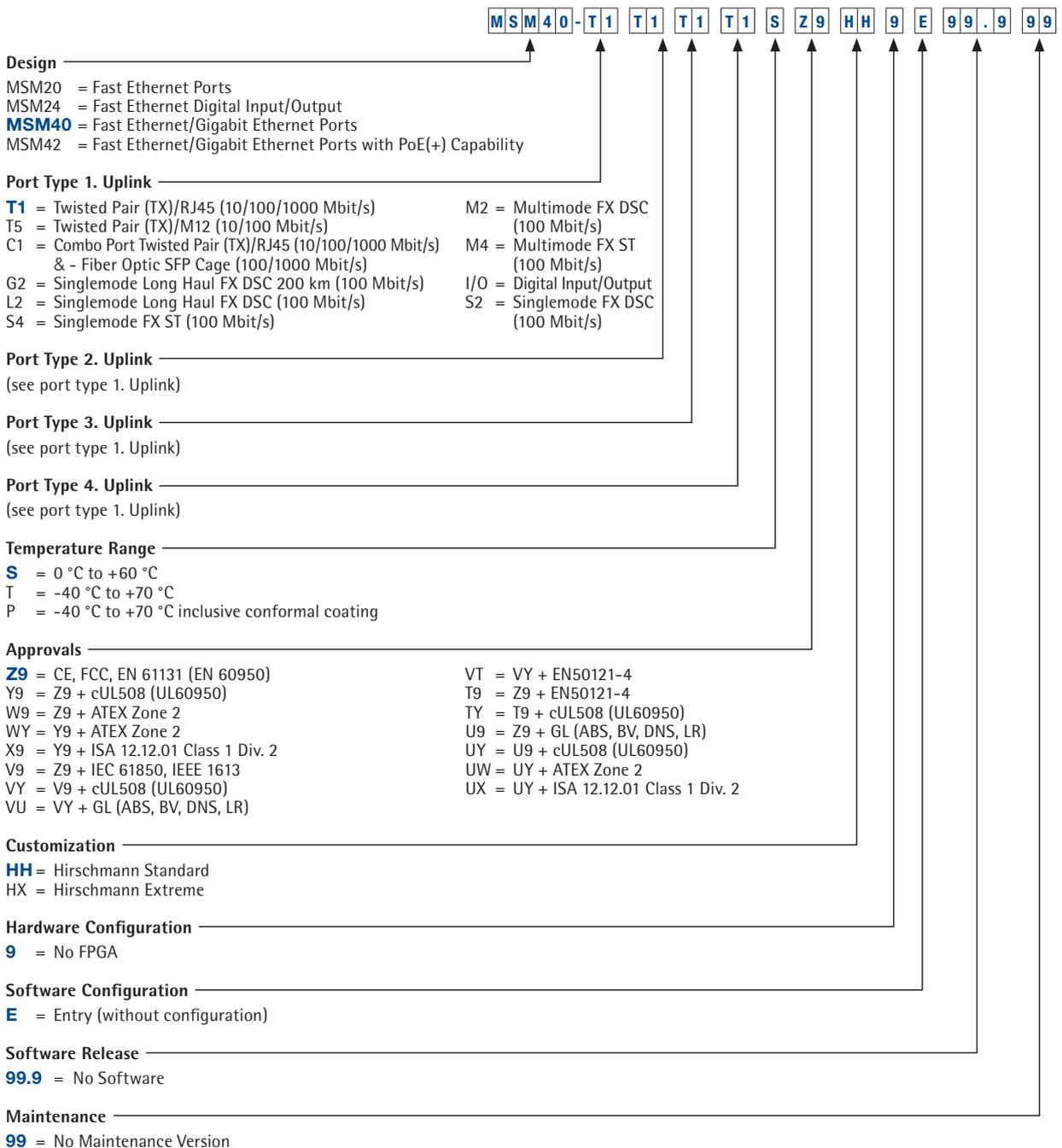
**NOTE:** The categories (Customization, Hardware Configuration, Software Configuration and Software Release) are optional.
