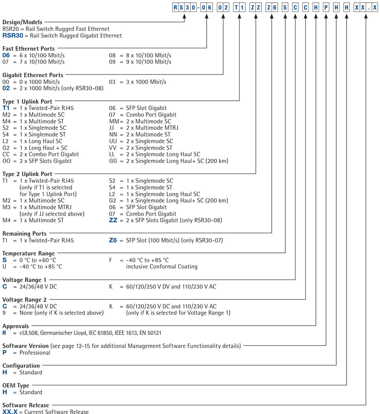
**NOTE:** The last three part number categories (**Configuration**, **OEM Type** and **Software Release**) are optional.
