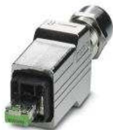
Push-pull connector (version 14), die-cast zinc, with RJ45 connector insert, 8-pos., with IDC fast connection technology, for 1 and 7-wire cores, 26 ... 24 AWG, for cable diameter of 5.5 mm ... 10 mm
