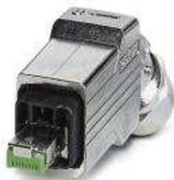
Push-pull connector (version 14), die-cast zinc, with RJ45 connector insert, 8-pos., with IDC fast connection technology, for 1 and 7-wire cores, 26 ... 24 AWG, for cable diameter of 5.5 mm ... 10 mm
