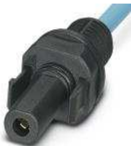
Photovoltaic connector, nominal current: 27 A, nom. voltage: 1500 V, connection method: Crimp, color: black. can only be released using a tool
