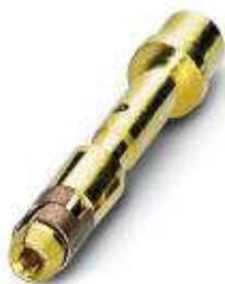
Crimp contact, turned, Single contact, Contact diameter: 1 mm, Crimp range: 0.06 mm²...0.25 mm²
