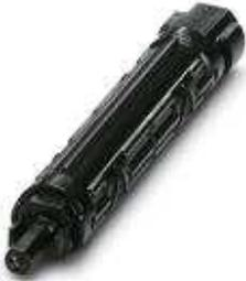
Fuse connector for protecting modules and devices in photovoltaic systems, black, SUNCLIX pin connector pattern, 1000 V/10 A, IP68 (24 h/2 m)
