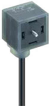
Actuator cordset, single-ended, valve connector according to DIN EN 175301-803, form A, with LED function indicator, suppressor diode voltage protection, connected protective earth
