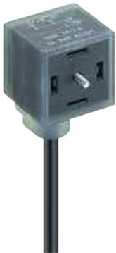
Actuator cordset, single-ended, valve connector according to DIN EN 175301-803, form A, with LED function indicator, varistor voltage protection, connected protective earth
