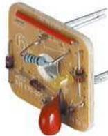
rectifier with protective circuit (varistor) and function indicator (LED)
