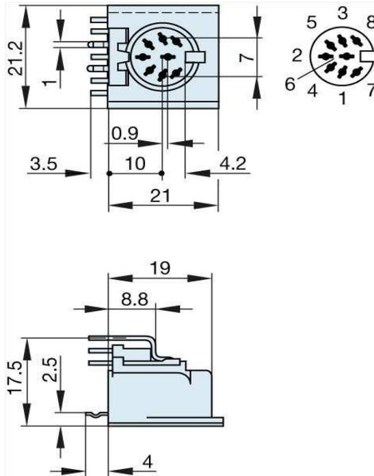
Arrangement of the soldering points on the components side
