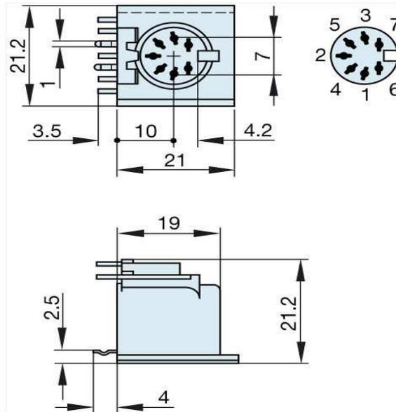
Arrangement of the soldering points on the components side
