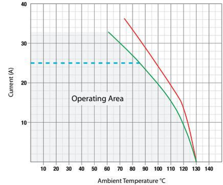
**7000 Series Current vs. Temperature Characteristics**
