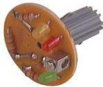
LED insert with 3 LEDs (green, red, yellow) to indicate operation conditions
