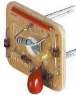
function indicator (LED) with freewheeling diode
