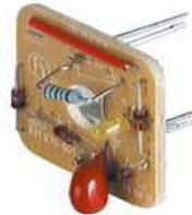
function indicator (LED) with freewheeling diode
