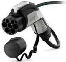
CHARX connect comfort, AC charging cable, with vehicle charging connector and open cable end, For charging electric vehicles (EV) with alternating current (AC) via GB/T vehicle charging inlets, with protective cap, GB/T, GB/T 20234.2-2015, GB/T 18487.1-2015, 32 A / 440 V (AC), housing: black, gray, PHOENIX CONTACT logo, cable: 7.5 m, black, straight, NOTE: Cable management may be required.
