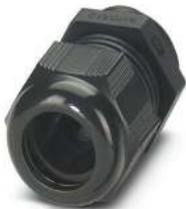
Cable gland, material for screw connection: PA, external cable diameter 11 mm . . . 17 mm, shielding: no, connecting thread: M25 x 1.5, color: jet black RAL 9005
