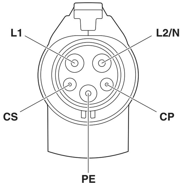
Pin assignment of the Vehicle Connector
