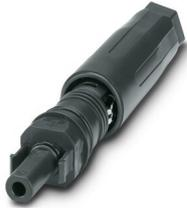
Photovoltaic connector, Range of articles: Sunclix, Connector, housing material: PPE, color: black, number of positions: 1, min. conductor cross section: 2.5 mm<sup>2</sup>, max. conductor cross section: 6 mm<sup>2</sup>, rated voltage: 1500 V DC, rated current: 35 A, Connection method: Spring-cage, Type of contact: Socket, min. cable diameter: 5 mm, max. cable diameter: 8 mm
