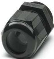
Cable gland, material for screw connection: PA, external cable diameter 15 mm .. 21 mm, shielding: no, connecting thread: M32 x 1.5, color: jet black RAL 9005
