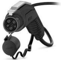
CHARX connect comfort, AC charging cable, with vehicle charging connector and open cable end, for charging electric vehicles (EV) with alternating current (AC) via type 1 vehicle charging inlets, with protective cap, with locking option for padlock, Type 1, IEC 62196-2, SAE J1772, PSE, 30 A / 250 V (AC), PHOENIX CONTACT logo, cable: 5 m, black, straight
