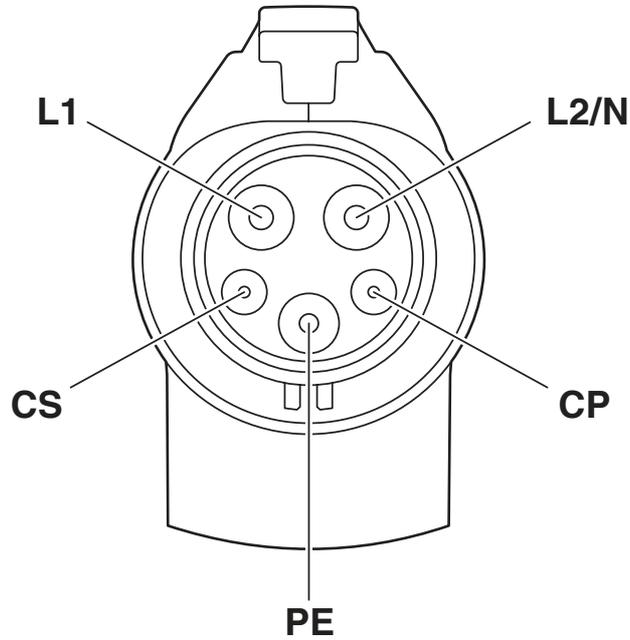
Pin assignment of the Vehicle Connector
