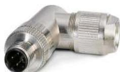
Data connector, Ethernet CAT5 (100 Mbps), 4-position, shielded, Plug angled M12, D, Insulation displacement connection, knurl material: Brass, nickel-plated, external cable diameter 4 mm ... 8 mm
