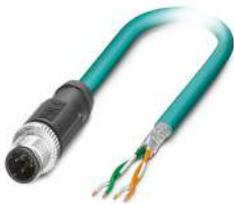
Network cable, Ethernet CAT5 (100 Mbps), 4-position, shielded, Plug straight M12, coding: D SPEEDCON / IP67, on free cable end, cable length: Free input (0.2 ... 40.0 m)
