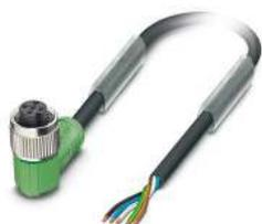
Sensor/actuator cable, 5-position, Variable cable type, free cable end, on Socket angled M12, coding: A, cable length: Free input (0.2 ... 40.0 m)
