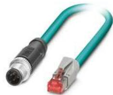
Network cable, Ethernet CAT5 (100 Mbps), 4-position, Variable cable type, shielded, Plug straight M12, coding: D SPEEDCON / IP67, on Plug straight RJ45 / IP20, cable length: Free input (0.2 ... 40.0 m)
