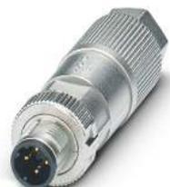
Data connector, PROFINET CAT5 (100 Mbps), 4-position, halogen-free, shielded, Plug straight M12, D, Insulation displacement connection, knurl material: Zinc die-cast, nickel-plated, external cable diameter 5 mm ... 9.7 mm
