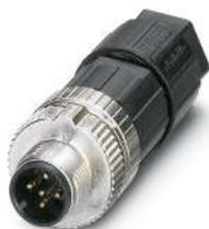
Connector, Universal, 5-position, unshielded, Plug straight M12, A, Push-lock spring connection, knurl material: Zinc die-cast, nickel-plated, external cable diameter 4 mm ... 8 mm
