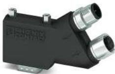
D-SUB plug, 9-pos., pin, assignment: 3, 5, 6, 8; two 35° cable entries M12 (B-coded). Bus system: PROFIBUS DP up to 12 Mbps. Termination resistor via separate M12 terminator.
