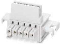
DIN rail connector, color: light grey, nominal current: 8 A (parallel contacts), rated voltage (III/2): 125 V, number of positions: 5, pitch: 3.81 mm, mounting: DIN rail mounting, locking: without, mounting: without, type of packaging: packed in cardboard, Item with gold-plated contacts, bus connectors for connecting with electronics housings, 5 parallel contacts
