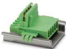
DIN rail connector, color: green, nominal current: 8 A (parallel contacts), rated voltage (III/2): 125 V, number of positions: 5, pitch: 3.81 mm, mounting: DIN rail mounting, locking: without, mounting: without, type of packaging: packed in cardboard, Item with gold-plated contacts, bus connectors for connecting with electronics housings, 5 parallel contacts
