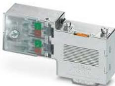
D-SUB connector, 9-pos., male connector, 90° cable entry, bus system: PROFIBUS DP up to 12 Mbps, termination resistor can be switched on via slide switch, pin assignment: 3, 5, 6, 8; IDC terminal block connection
