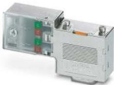
D-SUB connector, 9-pos., male connector, 90° cable entry, bus system: PROFIBUS DP up to 12 Mbps, termination resistor can be switched on via slide switch, pin assignment: 3, 5, 6, 8; screw connection terminal blocks
