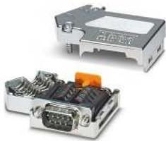
D-SUB connector, 9-pos., male connector, 35° cable entry, bus system: PROFIBUS DP up to 12 Mbps, termination resistor can be switched on via slide switch, pin assignment: 3, 5, 6, 8; screw connection terminal blocks
