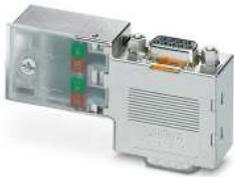
D-SUB connector, 9-pos., male connector, 90° cable entry, bus system: PROFIBUS DP up to 12 Mbps with PG D-SUB socket for connecting a programming device, termination resistor can be switched on via slide switch, pin assignment: 3, 5, 6, 8; screw connection terminal blocks
