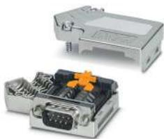
D-SUB connector, 9-pos., male connector, 35° cable entry, bus system: PROFIBUS DP up to 12 Mbps with PG D-SUB socket for connecting a programming device, termination resistor can be switched on via slide switch, pin assignment: 3, 5, 6, 8; screw connection terminal blocks
