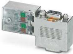
D-SUB connector, 9-pos., male connector, 90° cable entry, bus system: PROFIBUS DP up to 12 Mbps with PG D-SUB socket for connecting a programming device, termination resistor can be switched on via slide switch, pin assignment: 3, 5, 6, 8; IDC terminal block connection
