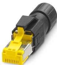
RJ45 connector, design: RJ45, degree of protection: IP20, number of positions: 8, 10 Gbps, CAT6<sub>A</sub>, material: Plastic, connection method: Insulation displacement connection, connection cross section: AWG 26- 24, cable outlet: straight, color: black, Ethernet
