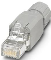
RJ45 connector, design: RJ45, degree of protection: IP20, number of positions: 4, 100 Mbps, CAT5, material: Plastic, connection method: Insulation displacement connection, cable outlet: straight, color: traffic grey A RAL 7042, PROFINET
