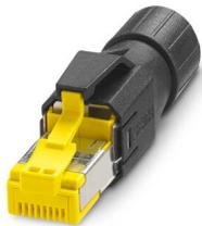
RJ45 connector, design: RJ45, degree of protection: IP20, number of positions: 8, 10 Gbps, CAT6<sub>A</sub>, material: Plastic, connection method: Insulation displacement connection, connection cross section: AWG 26- 24, cable outlet: straight, color: black, Ethernet
