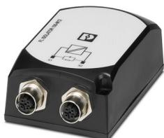
Passive network isolator for electrical isolation in Ethernet networks. For the protection of Ethernet devices against potential differences of up to 4 kV. Can be used for transmission speeds of up to 100 Mbps. Ethernet connection via two M12 sockets (D-coded).
