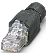
RJ45 connector, design: RJ45, degree of protection: IP20, number of positions: 8, 1 Gbps, CAT5, material: Plastic, connection method: Insulation displacement connection, connection cross section: AWG 26- 23, cable outlet: straight, color: black, Ethernet
