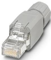
RJ45 connector, design: RJ45, degree of protection: IP20, number of positions: 8, 1 Gbps, CAT5, material: Plastic, connection method: Insulation displacement connection, connection cross section: AWG 26- 23, cable outlet: straight, color: traffic grey A RAL 7042, Ethernet
