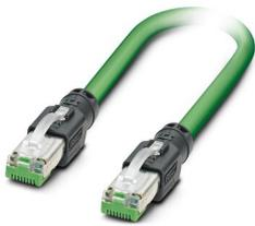
Patch cable, degree of protection: IP20, cable length: 2 m, number of positions: 4, 100 Mbps, CAT5, material: PA 6.6, PROFINET
