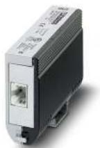
Surge protection in accordance with Class E<sub>A</sub> (CAT6<sub>A</sub>), for Gigabit Ethernet (up to 10 Gbps), token ring, FDDI/CDDI, ISDN, and DS1. Suitable for Power over Ethernet (PoE++ / 4PPoE) "Mode A" and "Mode B". RJ45 attachment plug with separate grounding cable and ground connection snap-on foot for NS 35 DIN rails.
