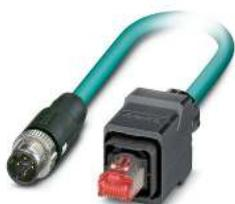
Network cable, Ethernet CAT5 (100 Mbps), 4-position, shielded, Plug straight M12, coding: D SPEEDCON / IP67, on Plug straight RJ45 Push Pull / IP67, cable length: 2 m
