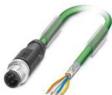
Network cable, PROFINET CAT5 (100 Mbps), EtherCAT® CAT5 (100 Mbps), 4-position, shielded (Advanced Shielding Technology), Plug straight M12, coding: D / IP67, on free cable end, cable length: 2 m
