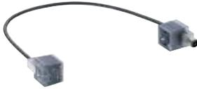
Double solenoid valve adapter (valve adapter with integrated M12 male receptacle connector), according to DIN EN 175301-803, form A, with LED function indicator and varistor for voltage protection, connected protective earth
