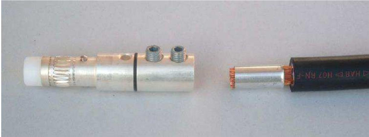
4. Select the appropriate reduction sleeves (see Table 1 below) and slide on in sequence over the exposed conductor stranding. All sleeves down to the size recommended for the cable in use should be used. i.e. for the 50mm<sup>2</sup> cable, the R120, R95, R70 and R50 sleeves should all be used. The sleeves fit inside each other to give a gradual reduction in diameter. The flared end of the sleeves should be against the cable insulation.
