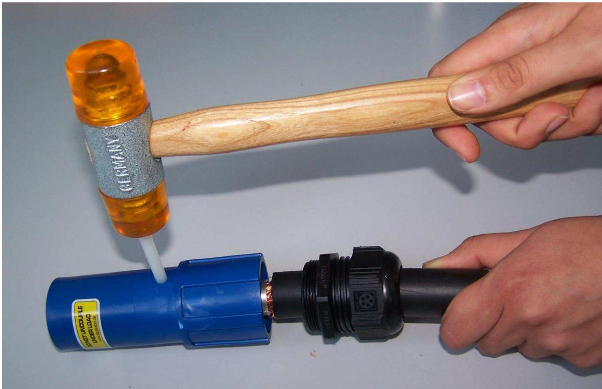
9. Ensure that the Retention pin is visible from both sides of the assembly after fitting and is flush/sub flush with the insulator.
