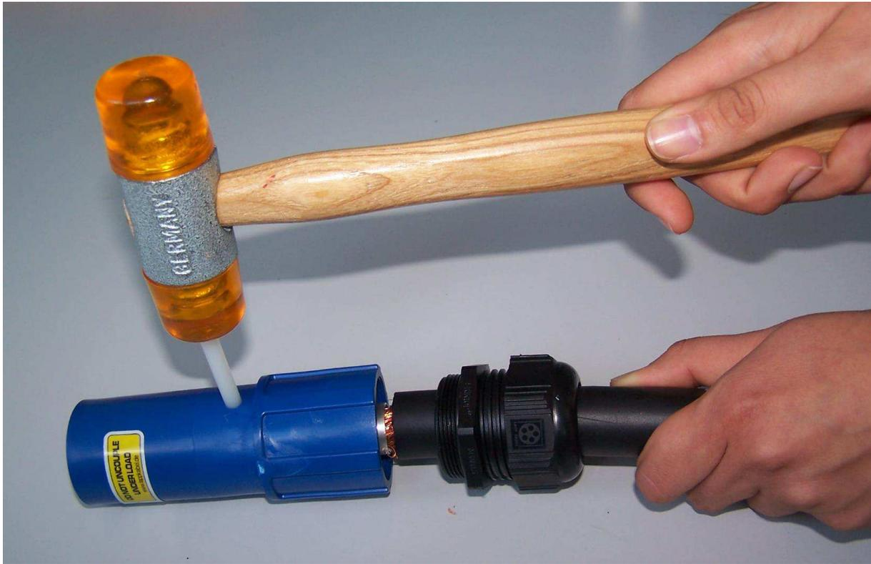
9. Screw the cable gland into the insulator, tightening to a torque of 13Nm minimum.
