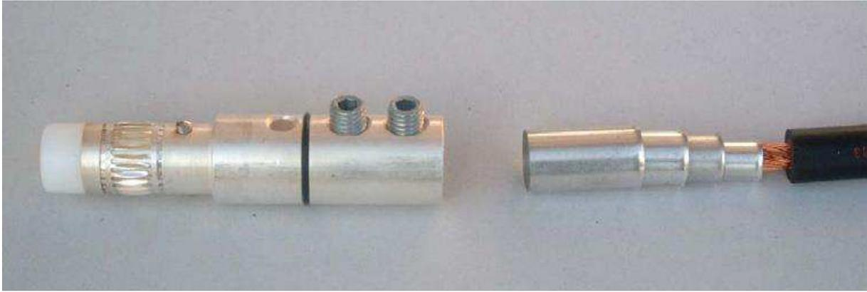
**5.** Slide the cable and reduction sleeves into the rear of the contact ensuring that they are fully seated inside of the contact. Using a 5mm A/F Allen key tighten the set screws to the appropriate torque setting.
